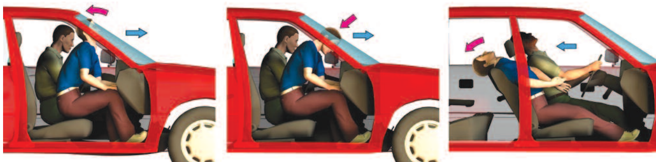
Fig. 1. Mechanisms underlying cervical spine injuries and basilar skull fractures in victims of motor accidents: A – hyperextension of the neck resulting from the face hitting the windscreen or front pillar of a vehicle; B – axial compression resulting from the crown of the head hitting interior elements of a vehicle; C – avulsion mechanism resulting from inertia force (operating in any direction – the figure presents only one of possible manners of inertial head displacement).
