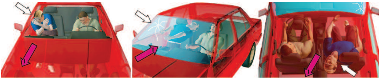
Fig. 4. The mechanism underlying an extension injury of the cervical spine resulting from a failure to fasten seat belts and missing the headrest in a situation of a corner-impact collision with a change of the inert force direction ( I ) in the second phase of the collision (the vehicle "bounces off" the obstacle).
